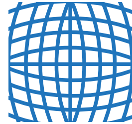
Barrel distortion Negative radial displacement
